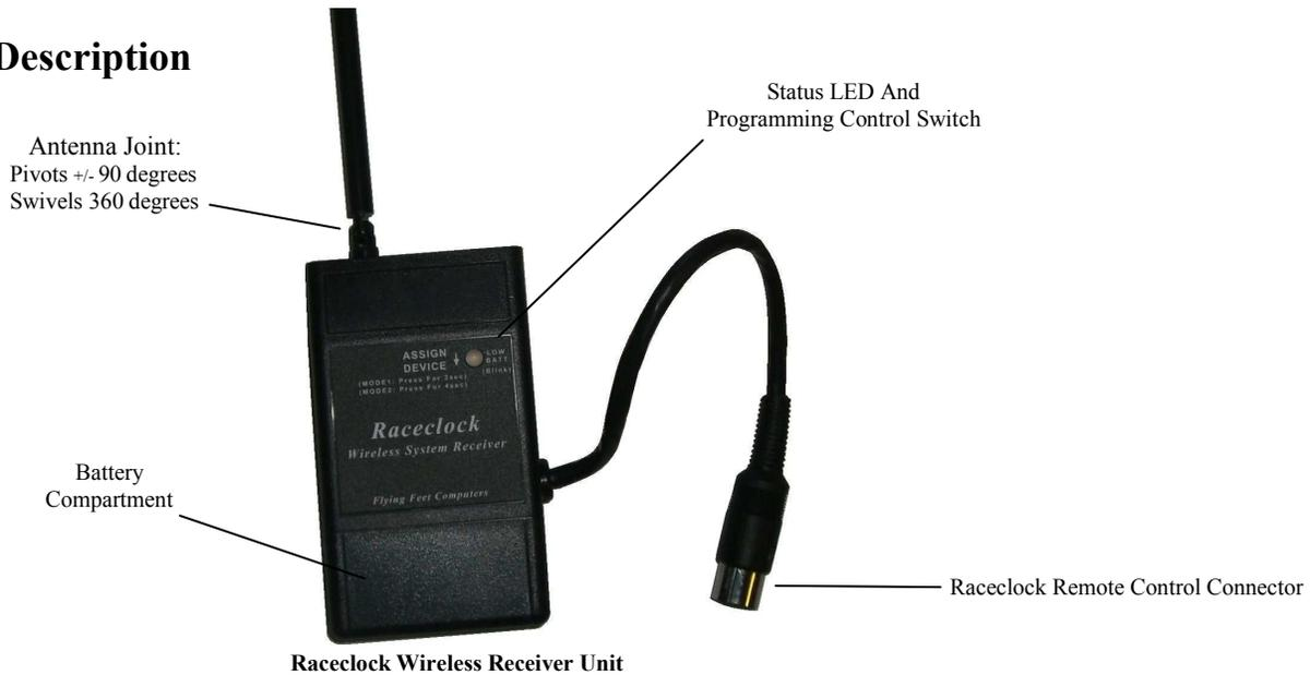
The Raceclock Wireless System Receiver Unit consists of a control box that features a Status LED/Programming Switch, a Front-Side Battery Compartment, an 8-pin Remote Control Connector and a 4” Antenna that can pivot vertically +/- 90 degrees or swivel horizontally 360 degrees.
